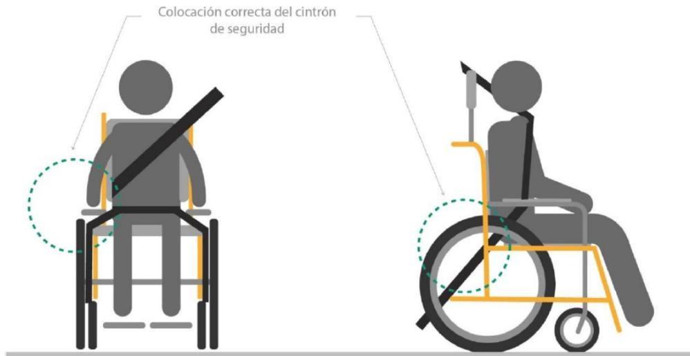
Para mayores detalles de las especificaciones se pueden consultar las normas *ISO 10542-1 Technical systems and aids for disabled or handicapped person – Wheelchair tiedown and occupant-restraint systems – Part 1: Requirements and test methods for all systems*, o la *ISO 7176-19 Wheelchairs – Part 19: Wheeled mobility devices for use as seats in motor vehicles*.
